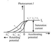
Changes in v causes changes in the maximum energy of the emitted photoelectrons and hence a change in the stopping potential.
