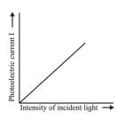
Collector at suitable +ve potential Frequency constant and above vo Intensity of light varied Current increases linearly with increase in Intensity
